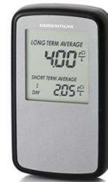
radon meter showing a reading of just over 2 pCi/L
